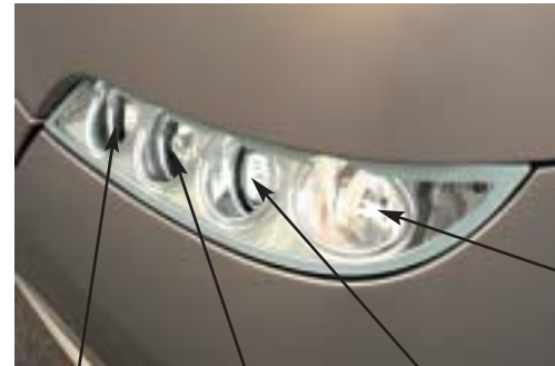
Auxiliary high beam Fog light Bi-Xenon® (low beam and high beam) Static bend lighting and position light
