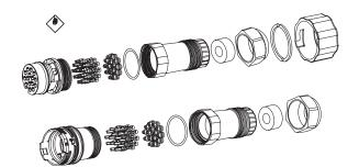
EasyConn connector/EasyConn mating connector With EasyConn connector set (15-pin, male) With EasyConn connector set (15-pin, female)
